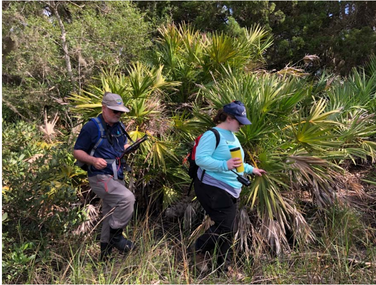
Kaitlyn Dietz and Jim Hunt walk the shoreline of the Guana Peninsula with an Arrow GNSS receiver to create a baseline map of erosion using ArcGIS Collector.
